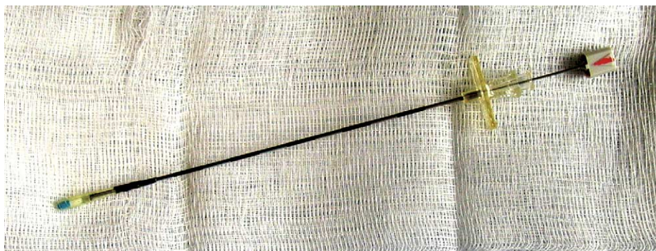
Fig. 1. Illustration of the pill pusher device constructed by the investigator for feeding the charcoal capsule to a rat. The device is composed of an epidural catheter with a plastic hollow tip cemented to the end of the catheter. The device is gently advanced into the esophagus past the esophageal sphincter and the capsule is released into the stomach after depressing the metal stylette.
